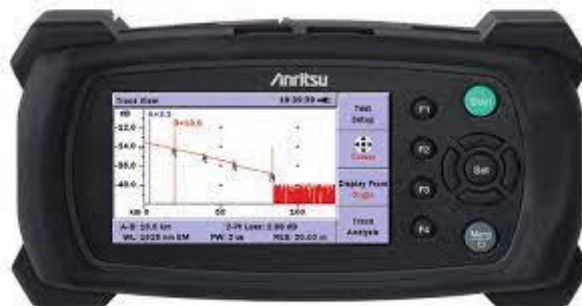
Rice. 3 Appearance of the MT9090 A analyzer Network Master c OTDR module
