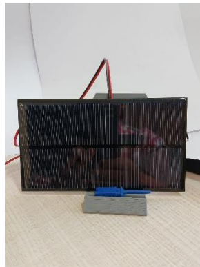
Figure 7. Li-Fi Demodulator, Sensor (Solar Cell, AK 150 X 85)
