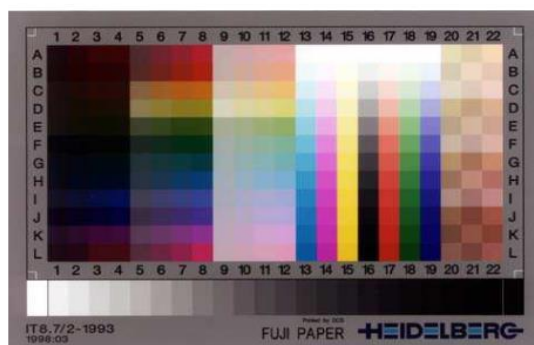
Fig.4. Test object (color scale), according to which you can select the desired shade of color
