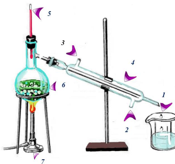
Fig. 3 Separation of volatile substances using the distillation method: collecting tank, 2- inlet of water cooler, 3- outlet of water cooler, 4- water cooler, 5- Thermometer, 6- process of driving liquid fraction, 7- tube heater
