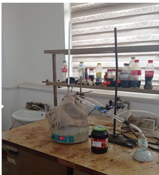
Fig. 3 Separation of volatile substances using the distillation method: collecting tank, 2- inlet of water cooler, 3- outlet of water cooler, 4- water cooler, 5- Thermometer, 6- process of driving liquid fraction, 7- tube heater
