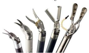
With one "hand" you can take the organ, move it back and fix it in the desired position. You can then activate another manipulator and continue working, all without an assistant. The manipulators have 7 degrees of freedom and are able to bend in ways that a surgeon's hands cannot.
