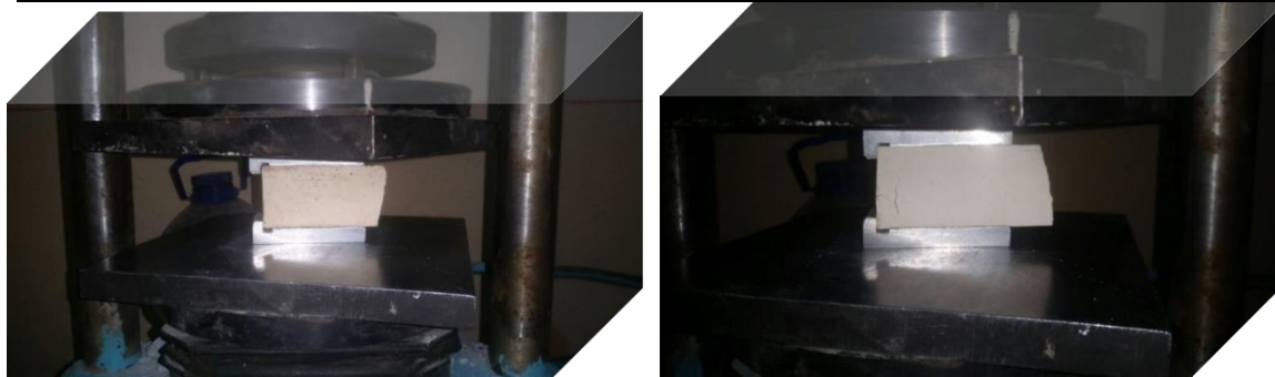
Fig. 7 determination of compressive strength limit
