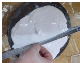
Figure 2. Determination of the normal thickness of gypsum paste
