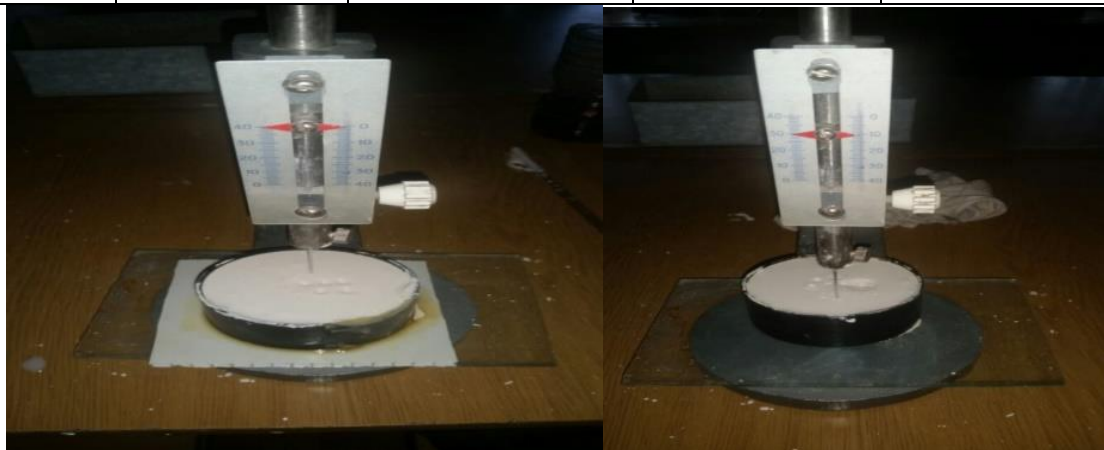
Fig. 4 Determination of the period of thickening of gypsum paste.
