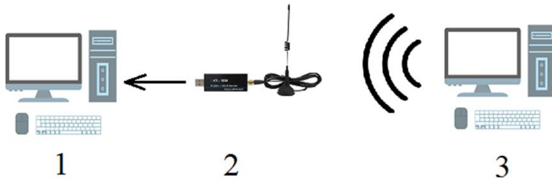
Figure 1. Block diagram for PEMI interception: 1-computer or laptop with special software for decoding SER radiation; 2-SDR receiver for receiving SER radiation; 3- SER source
