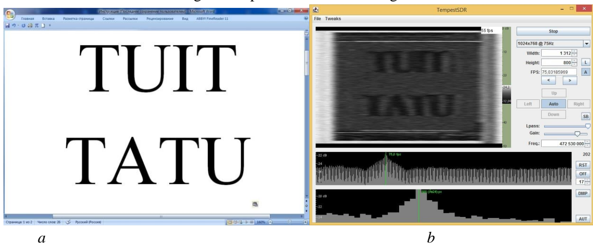
Figure 3. Demonstration of the image on (a) - on the monitor screen of the attacked computer; (b) - intercepted and reconstructed image.
