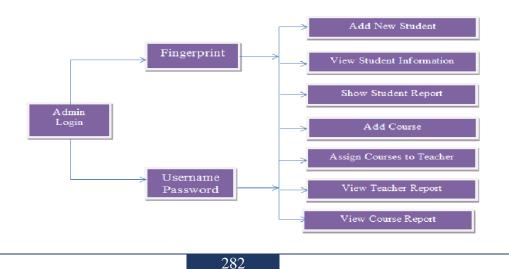
The system received the student's information by filling in the registration form and the student's fingerprints from the fingerprint scanner as input. The fingerprint scanner can read fingerprints of any or more fingers of both hands. The basic information was stored in the student profile table, and the fingerprints were stored in the template data table. In this template table, the key field is the student roll number, and all the templates have differed by this roll number.
