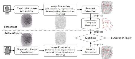
The block diagram in the pictures the methodological steps for developing the proposed attendance system. The proposed approach has five major components, such as (i) user and device interface, (ii) data acquisition with fingerprints, (iii) fingerprint processing, (iv) taking class with fingerprint verification, and (v) attendance report generation.
