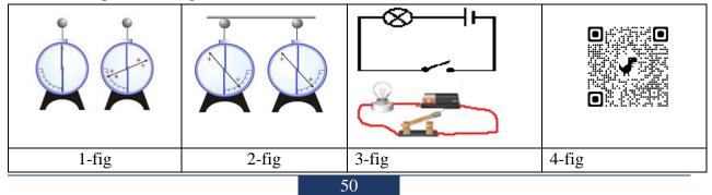
**3-experience**. The chain shown in Figure 3 is assembled. The chain consists of a current source, a light bulb and a switch. With a key connection in the chain, the light bulb lights up (fig. Readers will be asked to explain the cause of the light bulb burning. Readers' opinions are listened to. Then it is recommended to view the animation of the experiment by QR code (fig. 4)
