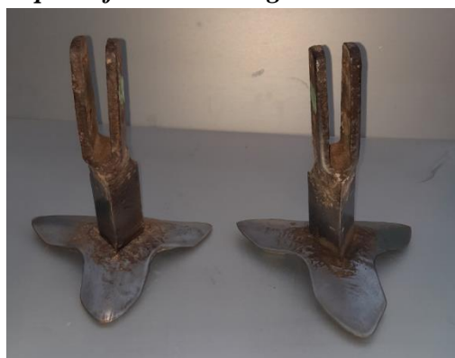
9-Figure The condition of the experimental paw before and after the field test.
