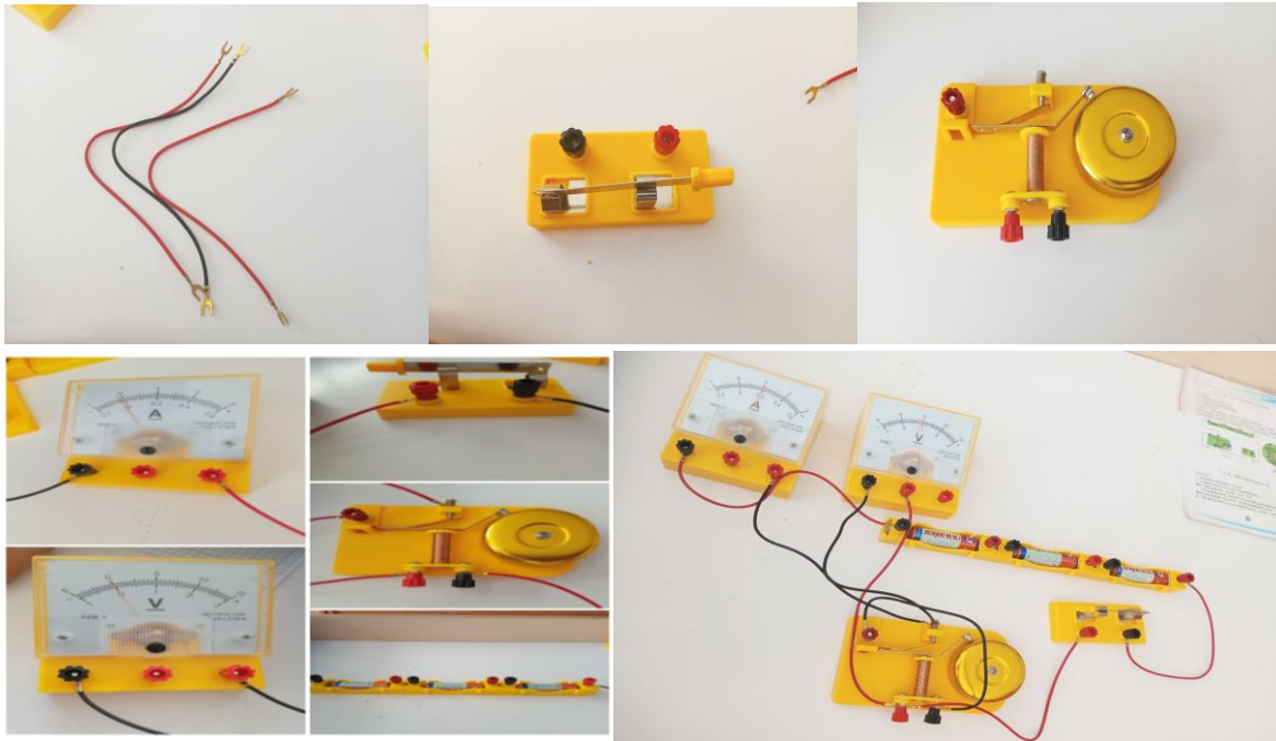
Assembly of the simplest radio
