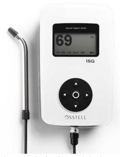
The index of mutual connection between the implant and the bone surrounding it is the main factor determining the stability of the implant. A sensor connected to the instrument transmits the resonance frequency value through a signal, and its result is displayed on the screen. The so-called Implant Stability Quotient (ISQ) has a value from 1 to 100.
