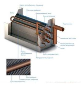
During operation, water heaters can withstand large temperature changes. That is: 70-110°C. For this type of heater to work well, the water circulating in the system should be heated to a maximum of 180°C. In the hot season, the heater can also be used as a cooler to cool the rooms of the building.
