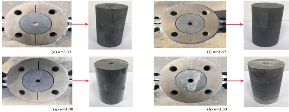
Fig. 5. Blasted iron ore under different decoupling charge coefficients.
